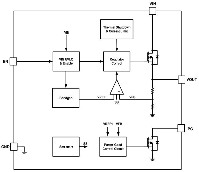
Figure 18. Functional Block Diagram
