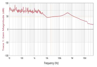
Figure 16. PSRR vs Frequency at lout=10mA, Cout=22uF
