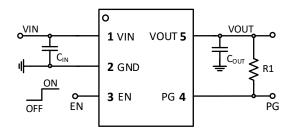
Figure 25. SCT71203 Typical Application Schematic
