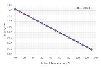
Figure 31. Maximum Allowed Power Dissipation vs Ambient Temperature, SOT23-5,T\_J  $\leq$  150°C
