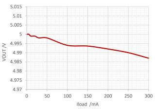
Figure 10. Output Voltage vs Output Current
