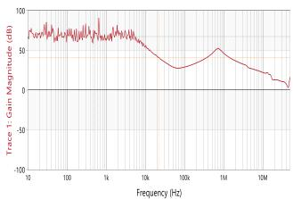
Figure 13. PSRR vs Frequency at lout=100mA, Cout=4.7uF
