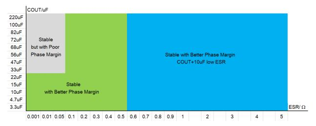
Figure 28. SCT71203 Stability vs Output Capacitor
