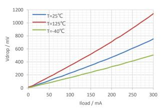
Figure 6. Dropout Voltage vs Output Current
