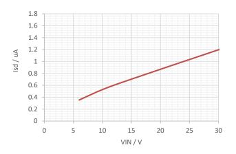
Figure 5. Shutdown Current vs Input Voltage
