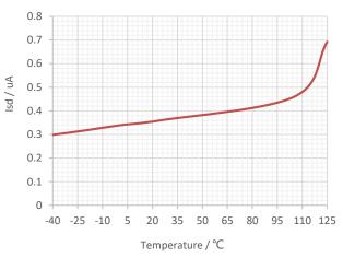
Figure 4. Shutdown Current vs Ambient Temperature
