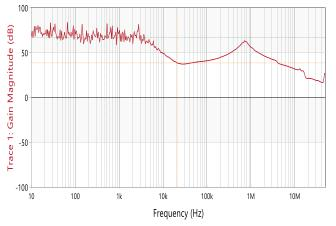
Figure 12. PSRR vs Frequency at Iout=10mA, Cout=4.7uF
