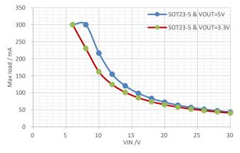
Figure 30. Maximum Output Current vs Input Voltage,  $SOT23\text{-}5, T_J \leq 150^\circ\text{C}$
