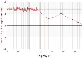
Figure 15. PSRR vs Frequency at lout=100mA, Cout=10uF
