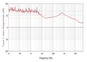
Figure 14. PSRR vs Frequency at Iout=10mA, COUT=10uF
