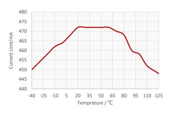
Figure 11. Output Current Limit vs Ambient Temperature
